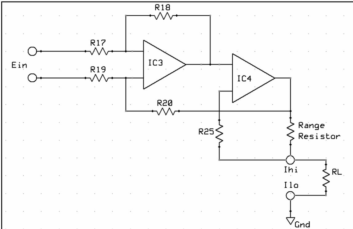
Figure 3 Transconductance Amplifier
